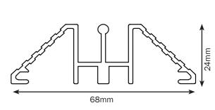
This track can be installed on a flush floor without creating a tripping hazard
