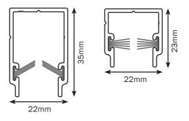
The Standard Track is designed for maximum mesh retention in most applications whilst the Small Track has been introduced for internal shading where wind is not a factor
