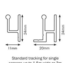
Standard tracking for single screens up to 1.5m wide or 3m for a double screen
