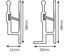
Mesh retention tracking for single screens over 1.5m wide or over 3m for a double screen
